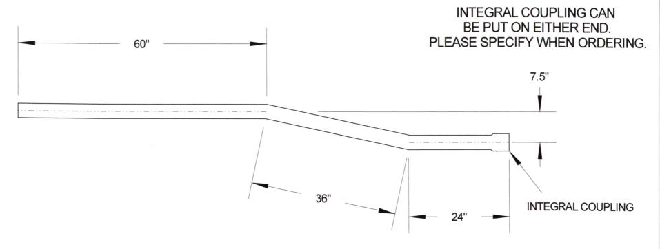
STANDARD OFFSETS CAN BE MADE FROM S/40 OR S/80 PVC IN 2", 3", OR 4" IPS SIZES (OTHER SIZES AVAILABLE BY REQUEST)
